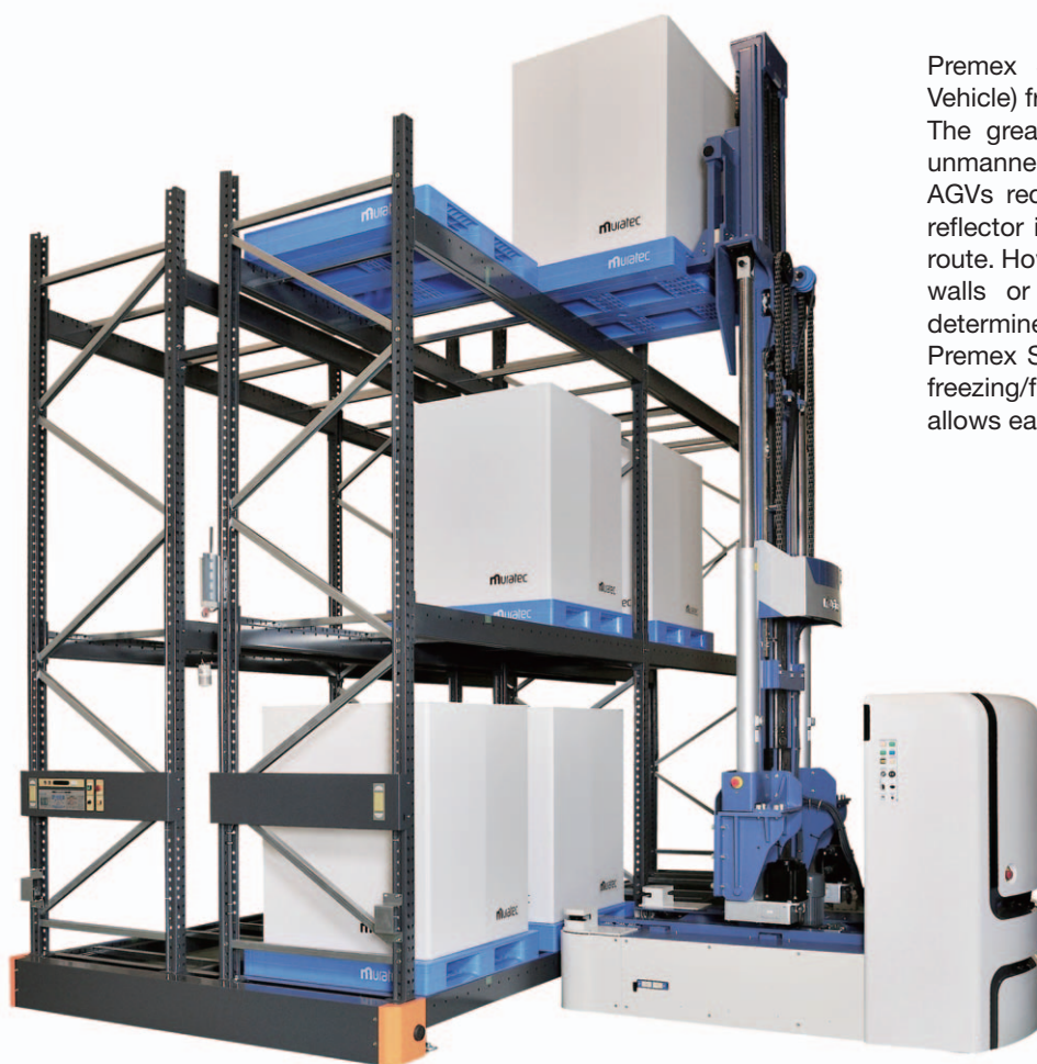
Compatible with mobile rack transfer. Flexible travel in small spaces by multi-drive.
